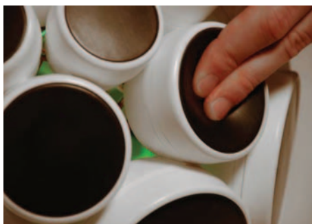
AlphaSphere is made up of 48 pressure-sensitive pads that form a self-supporting spherical structure
